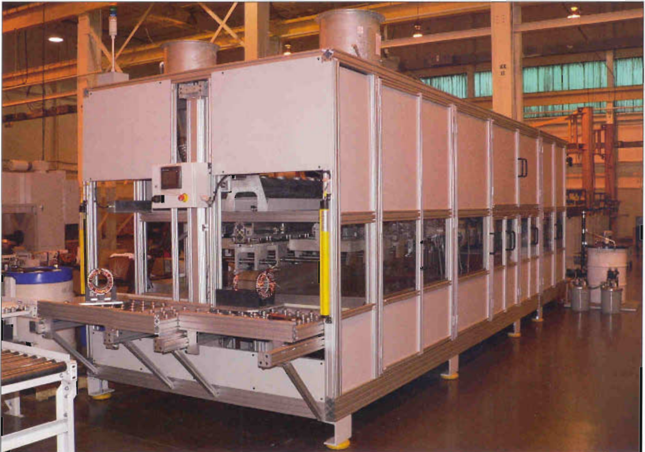
Multi-station linear indexing machine showing the load / unload station and operator's console
